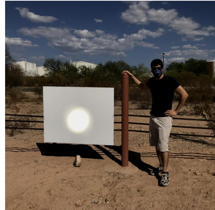
Solar disc image obtained at 2:30 pm, screen 40 m to the East, 62° AOI
